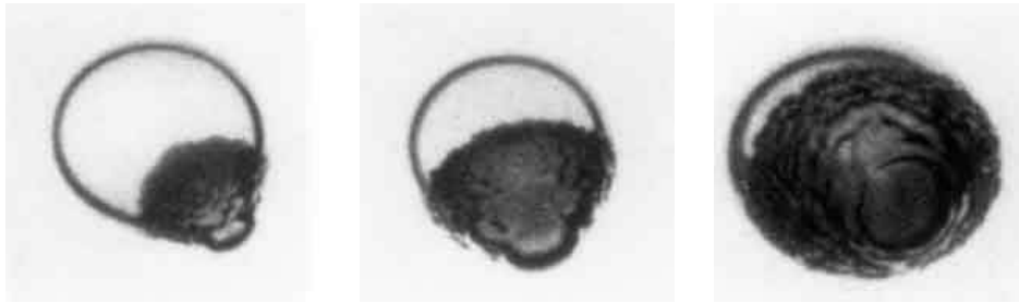
Figure 7.8: Typical photographs of a rapidly growing bubble in a droplet of superheated ether suspended in glycerine. The bubble is the dark, rough mass; the droplet is clear and transparent. The photographs, which are of different events, were taken 31, 44, and 58 \mu s after nucleation and the droplets are approximately 2mm in diameter. Reproduced from Frost and Sturtevant (1986).
