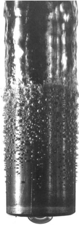
Figure 7.14: The evolution of convective boiling around a heated rod, reproduced from Sherman and Sabersky (1981).
